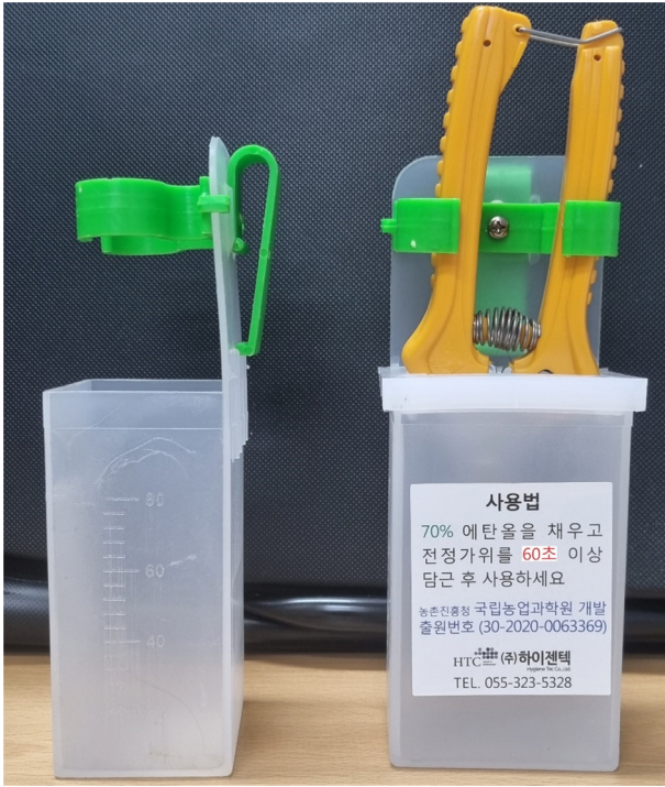
Fig. 4. Pruning scissor disinfection cradle.
